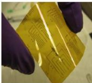
Figure 2: Ambipolar, bottom contact pentacene transistors fabricated on Kapton® and their device characteristics.
